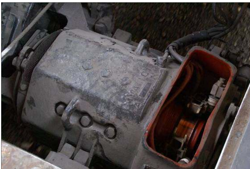
40 Horse Power, 600 volt DC, Electric Motor as used on the trams on the Dockline Tramway.
